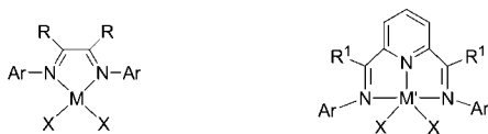
Scheme 1. N-ligand-stabilized late-transition-metal olefin polymerization precatalysts (for instance: M = Ni, Pd; M' = Fe, Co; X = Cl; R = H; R 1 = CH 3 ; Ar = 2,6-diisopropylphenyl).
